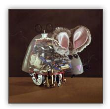
**1978** Micromouse, called "Moonlight Special," took 500 voluntary hours to assemble. It was a self-contained robot that used microprocessor technology to solve complicated mazes.
