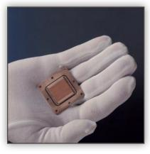
**1999** Researchers developed the award-winning MicroHeater, a palm-sized combustion unit that weighed less than .2kg (5 oz.). The technology could provide heat for portable personal heating and cooling devices, in-line water heaters, fuel cell systems, and indoor heating systems.
