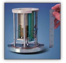
**1999** The award-winning Electrodynamic ion Funnel designed at PNNL significantly improved the sensitivity of certain mass spectrometry tools and other analytical instruments. Mass spectrometry is used in environmental, biotechnology and drug applications, as well as in medical, biological and other broad areas of research.
