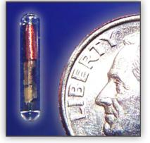
**1998** PNNL improved radio-frequency identification tags that were used to track and monitor everything from clothing to pharmaceutical products to computer equipment. These tags currently are used by the U.S. military.
