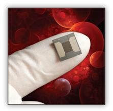
**2010** Molecular traces can be telltale signs of explosives in a briefcase or progressing human disease. Revolutionary ion mobility separations in a microchip, developed at Owlstone Nanotech and PNNL, dramatically improve the ability to rapidly detect specific molecules in complex samples.
