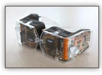
2014 The Glyph™ is a threedimensional headset display that contains PNNL-developed virtual retinal technology that's easier to read. The technology was commercialized for military applications to improve the sight of soldiers in dark battlefields and aid with piloting armored or unmanned vehicles. It also shows promise for applications such as surgery and virtual training.
