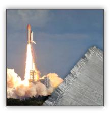
**1989** Advanced ceramic fabric materials developed at PNL helped in space exploration. Ceralite<sup>™</sup> materials, made from continuous fibers of metallic oxides or other low-density materials, were used on space shuttle flights to significantly reduce the mass and weight of heat radiators, piping, and other spacecraft components.
