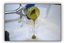
**2013** A continuous chemical process developed by PNNL engineers produces useful crude oil minutes after they pour in harvested algae. With additional conventional refining, the crude algae oil is converted into aviation fuel, gasoline or diesel fuel.
