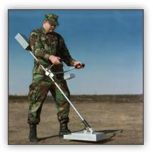
**2000** PNNL engineered the Timed Neutron Detector, an award-winning technology, which quickly and easily detects metallic and non-metallic landmines.
